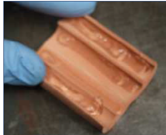
Open block and apply GB Pro Sealant to inside surfaces.
