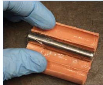
Insert Blank plug if required spread sealant over all internal surfaces.
