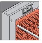
**IO** Build up frame repeating the process described in steps 2-9. In this example 2 more cables have been added using other block sizes.
