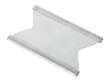
To be placed between each row of blocks. Stayplates make installation simple, increase stability and anchor blocks within the frame. Stayplates are available in galvanized or stainless steel.
