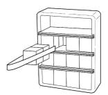
2. Ensure the tweezers blades protrude at least 35 mm outside the block. Insert the tweezers blades in the frame.
